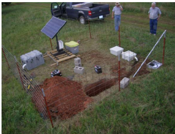
Installation of in situ sensors at MOISST. Image credit: Michael Cosh [USDA]
