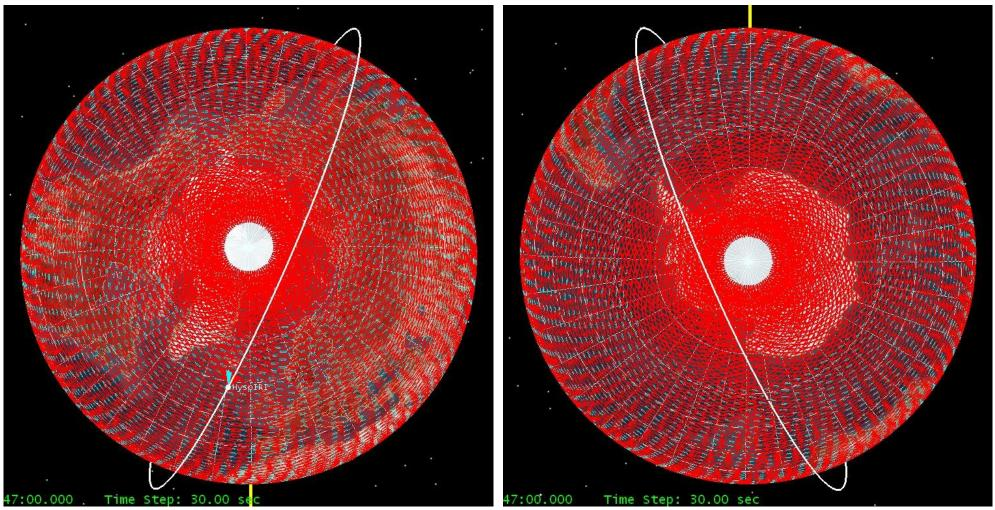
HyspIRI's nominal mid-morning (10:30 AM) crossing time is on a descending orbit (N-to-S) pass. Hence the observatory passes over sunlit terrain while descending east of the North Pole and while approaching west of the South Pole. TIR coverage is similar at both poles. (Ground tracks of sun-synch. orbits cannot pass directly over the poles.) Because the VSWIR sensor relies on reflected illumination, it can collect data from well-illuminated surfaces at higher latitudes in the north.
