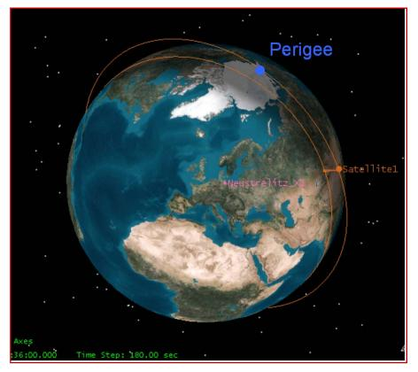
Sun-synchronous, 11:00 LTDN LEO – reference altitude 653km 3 axis stabilized platform with OCS mass 850 kg / power 550 W avg. 512 Gbit mass memory / 320 Mbit/s Xband science data downlink 4 day global accessibility ( 30 off-nadir) 4 day target revisit capability up to 50 data takes per day / total length 5000km
