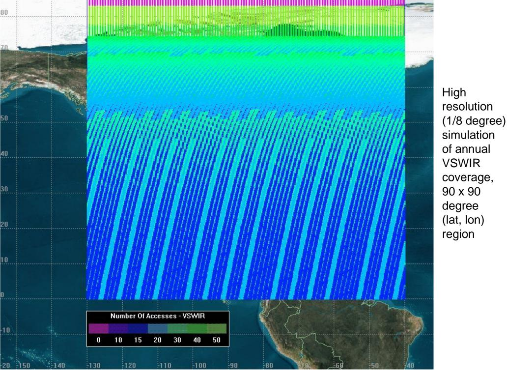
Nominal orbit: av. alt. 626.8 km, incl. 97.8°. VSWIR spectrometer FOV: 2.8° E, 10.8° W (60 m pixel GSD at nadir, 2480 cross-track pixels). R.G. Knox, NASA GSFC, Biospheric Sciences Branch, Code 614.4. Simulated with STK v9.2, August 17, 2010. Note aliasing at high latitudes.
