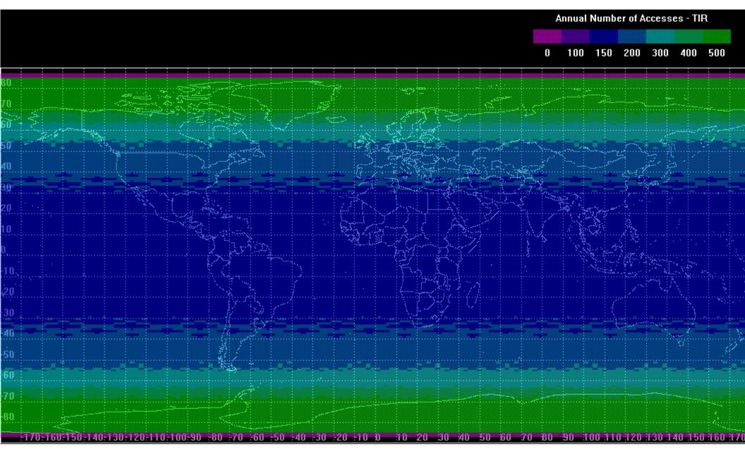
Nominal orbit: average alt. 626.8 km, inclination 97.8°. TIR imager FOV: +/- 25.46° (60 m pixel GSD at nadir, 9272 cross-track pixels). R.G. Knox, NASA GSFC, Biospheric Sciences Branch, Code 614.4. Simulated with STK v8.1.3, March 7, 2010. Plotted May 3, 2010. Annual TIR imaging opportunities in a 19/5-day repeat HyspIRI reference orbit Swath: 50.92°, symmetric about nadir. Sampled using a 1 by 1 deg. coverage.
