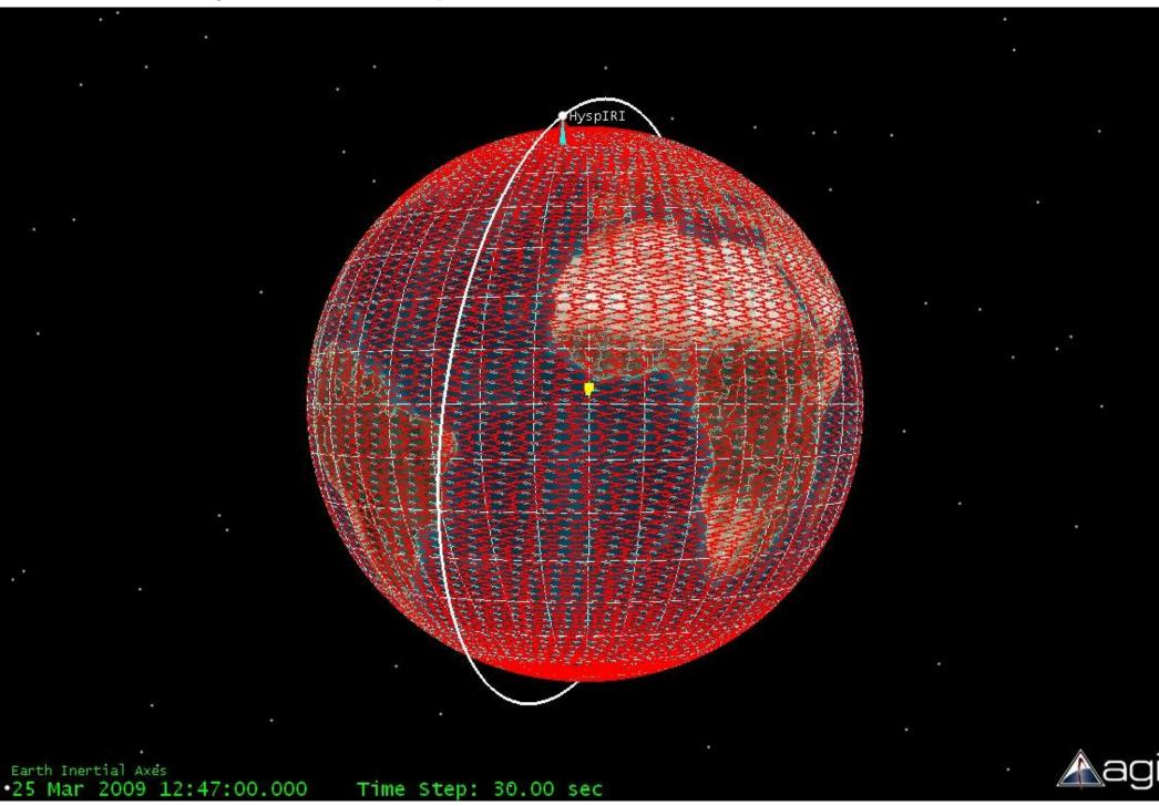
R.G. Knox simulation with STK v9.2. Orbit: alt. 626.8 km, inclination: 97.8°. Earth graphics courtesy of Analytical Graphics Inc.
