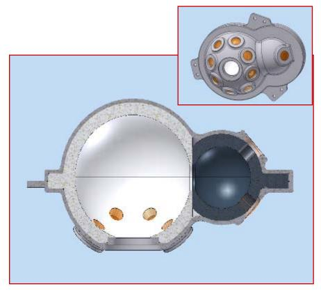
Radiometric stability check: "integrating sphere with sources at different levels" Sources: 10W Halogen lamps white high power LEDs Coupling to spectrometers via imaging optics Different levels by driving varying currents
