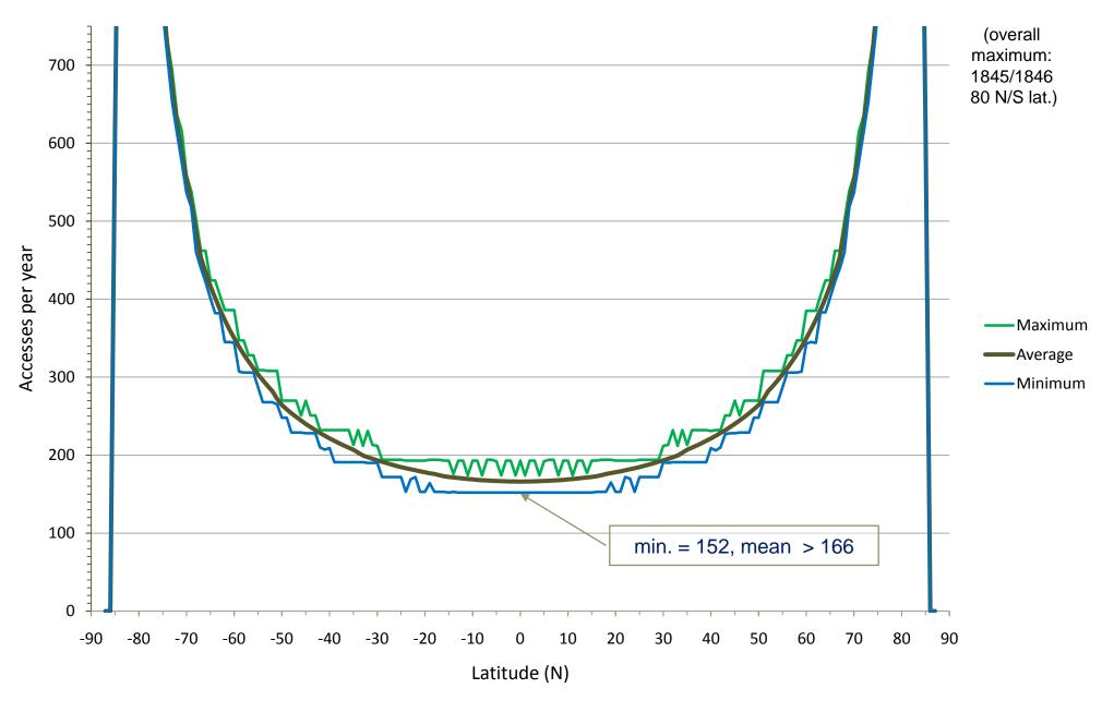
Nominal orbit: average alt. 626.8 km, inclination 97.8°. TIR imager FOV: +/- 25.46° (60 m pixel GSD at nadir, 9272 cross-track pixels). R.G. Knox, NASA GSFC, Biospheric Sciences Branch, Code 614.4. Simulated with STK v8.1.3, March 7, 2010.
