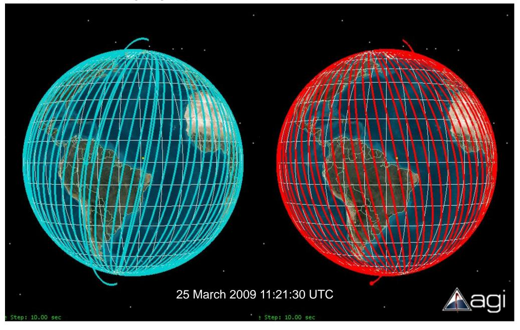
R.G. Knox simulation with STK v8.1.3. Orbit: alt. 626.8 km, inclination: 97.8°. Earth graphics courtesy of Analytical Graphics Inc.
