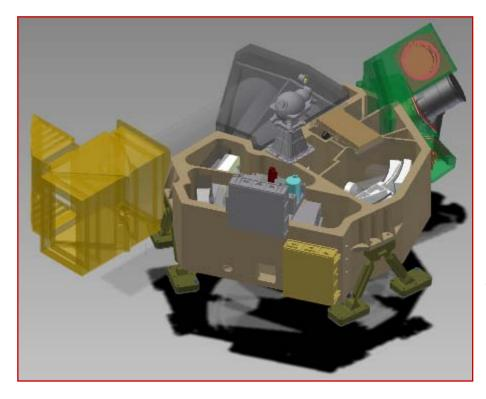
Polished NiP coated Aluminum mirrors Monolithic Aluminum structure Quasi-isostatic mounting to platform Starcameras attached to IOU for pointing knowledge Redundant SWIR FPA due to cryocooler without flight heritage Gravity release < 5µm – opt. elements Eigenfreq. > 100 Hz Active thermal stabilization to 21 C <u>+</u> 1K
