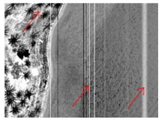
Striping in Pushbroom sensor data (MNF-transformed)
