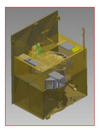
Total Weight: ca. 850 kg Aver. Power: 450 W 512 Gbit mass memory 3 axis stabilized platform Pointing Stability: 1,5 m / 4 ms Pointing Knowledge: 100 m 30 off nadir pointing for observation Hydrazine propulsion system for orbit maintenance & disposal 320 Mbit/s X-Band science data downlink Lifetime in Orbit: > 5 years
