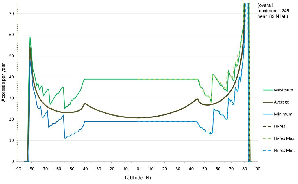
Nominal orbit: av. alt. 626.8 km, incl. 97.8°. VSWIR spectrometer FOV: 2.8° E, 10.8° W (60 m pixel GSD at nadir, 2480 cross-track pixels). R.G. Knox, NASA GSFC, Biospheric Sciences Branch, Code 614.4. Simulated with STK v9.2, Aug. 20, 2010.; hi-res subset Aug. 17.
