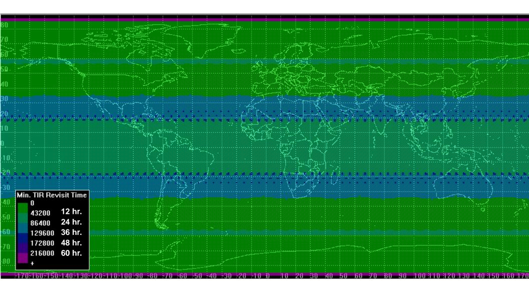
Nominal orbit: alt. 626.8 km, incl.: 97.8. TIR sensor FOV: +/- 25.46 (60 m pixel GSD at nadir, 9272 cross-track pixels). R.G. Knox, NASA GSFC, Biospheric Sciences Branch, Code 614.4. Simulated with STK v8.1.3, March 20, 2010. Plotted May 3, 2010.
