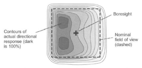
Figure 4.2. Example of a typical actual sensor 2-D response function for a sensor having a nominally square.
