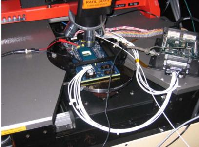
Wafer probe station. Wafer is currently being testing at nearly the required readout speed and shows as-expected noise and power performance as well as register functionality.
