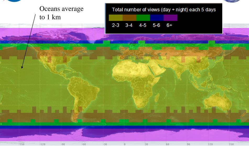
Nominal orbit: average alt. 626.8 km, inclination 97.8°. TIR imager FOV: +/- 25.46° (60 m pixel GSD at nadir, 9272 cross-track pixels).
