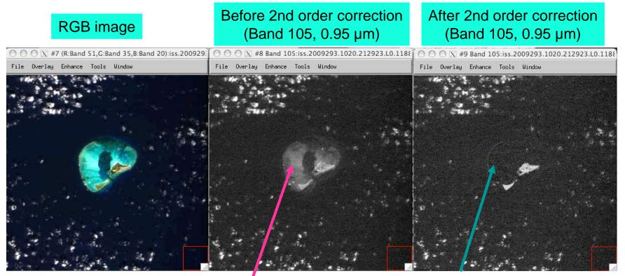
The bright features result from the 2<sup>nd</sup> order light of a visible channel
