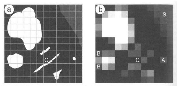
Figure 7.10. Schematic of the visible waveband view reflected from a region of partially cloudy sea. (a) As seen by a very fine resolution detector, with a coarse grid of  $12 \times 12$  cells superimposed. (b) As it appears in the coarse pixels image.
