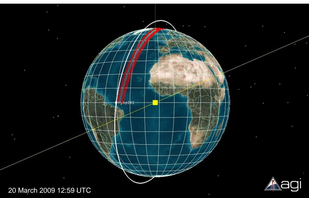
Orbital inclination (97.9) represents the angle between the Earth's equatorial plane, and the orbit plane, measured (by convention) at an ascending node.
