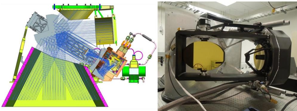
Figure 4. (left) Design of ECOSTRESS TIR Push-whisk scanning system covering a wide field of view with an 8 band SWIR to TIR sensor. (right) Developed, aligned and qualified PHYTIR push-whisk system with TIR full range multi-band detector array.
