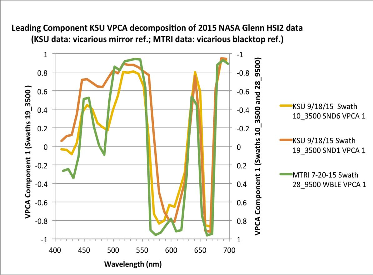
Figure 8. Spectral signatures of potentially toxic cyanobacteria in Sandusky Bay and the Western Basin of Lake Erie extracted from images swaths collected by the 2<sup>nd</sup> generation, NASA Glenn Hyperspectral Imager (HSI2) during the summer of 2015. The signals are obtained through a varimax-rotated principle component analysis of the derivative spectra correlation matrix [Source: NASA Glenn Lake Erie HAB Technical report, 2016].
