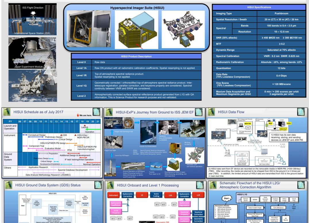
HISUI GDS consists of the four subsystems: • Observation and Planning Subsystem (OPS) • Product Generation Subsystem (PGS) • User Interface Subsystem (UIS) • System Integration Subsystem (SIS)
