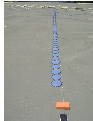
70 point facets create the linear target
