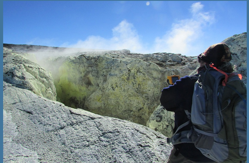
Measuring radiant temperature at active fumarole site (photo courtesy of USGS-HVO)
