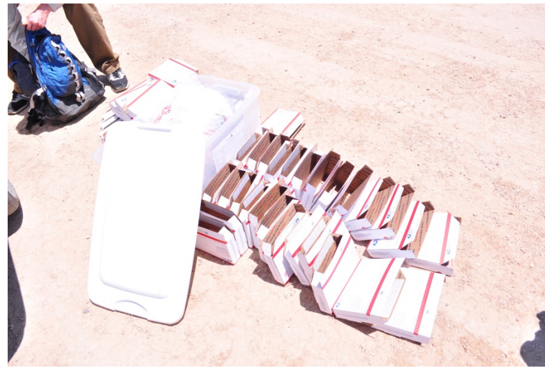
Soil sampling boxes for surface emissivity measurements
