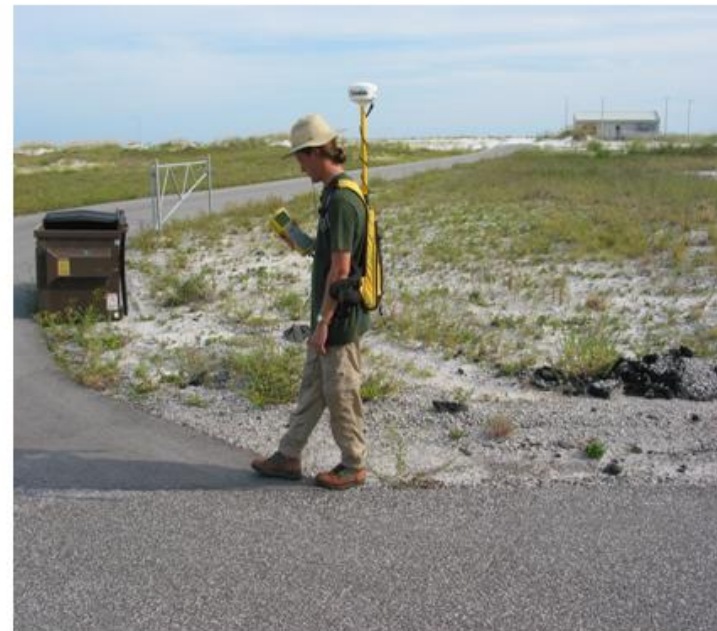
GPS measurements for geolocation information
