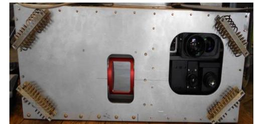
Designed to study composition, structure, and function of terrestrial surfaces using; scanning LiDAR, Hyperspectral & Thermal infrared imaging.
