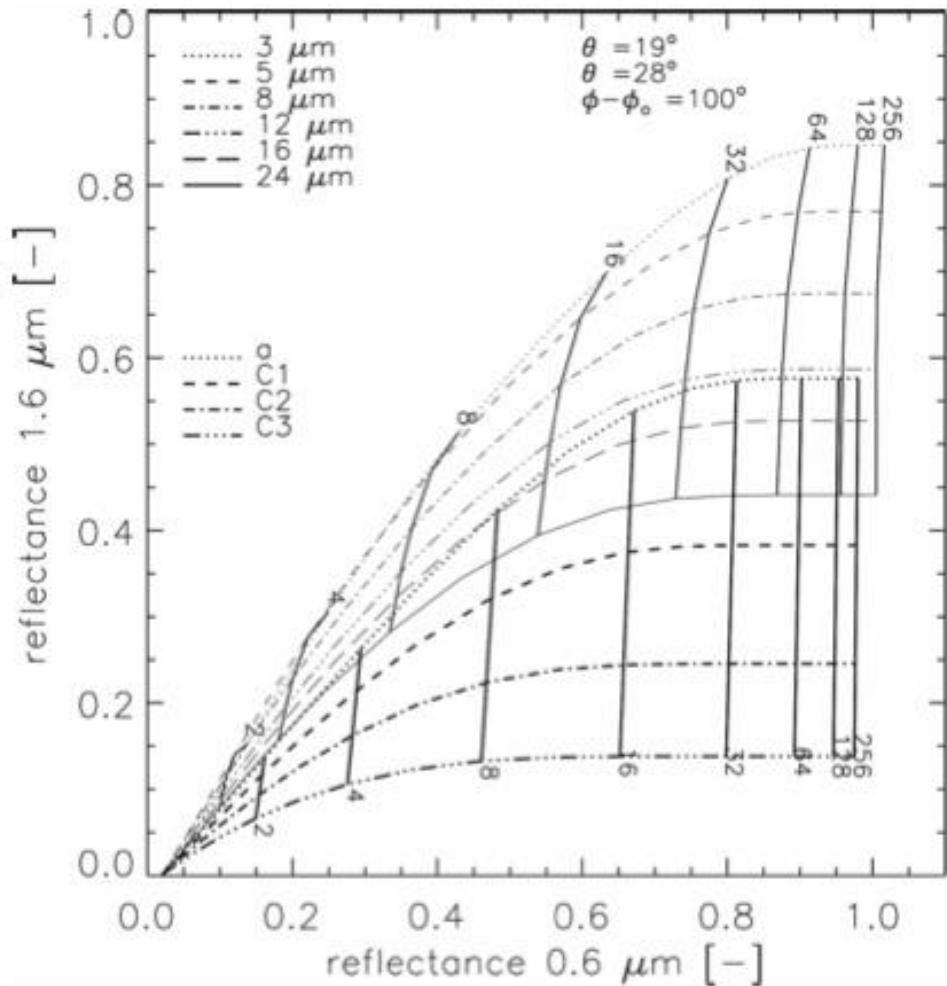
FIG. 2. Modeled 0.6- and 1.6- $\mu\text{m}$  reflectances for  $\theta_0 = 19^\circ$ ,  $\theta = 28^\circ$ , and  $\phi - \phi_0 = 100^\circ$ . Cloud optical thickness is denoted by various vertically oriented lines, and the effective radius is denoted by horizontally oriented lines. Water particles are represented in the top part of the graph, and ice particles are shown in the bottom part.
