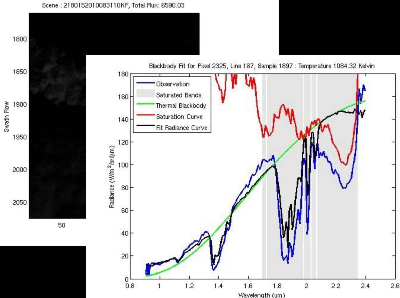
Fit to spectrum to quantify thermal emission
