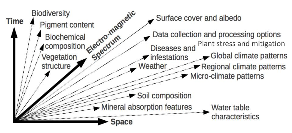
Spectral data provide the basis for understanding plant or ecosytem functioning due to well-known — and some not so well understood — optical properties associated with leaf/canopy structure, biochemistry, physiology, etc. In situ spectral data are critical to scaling to remote sensing imagery
