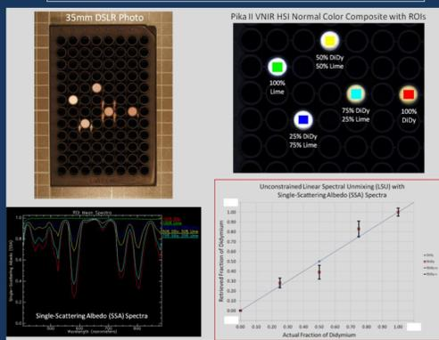
Mixtures of pure materials can be examined and used to study non-linear mixing. The resulting data set can then be used to develop predictive models. Ref 2
