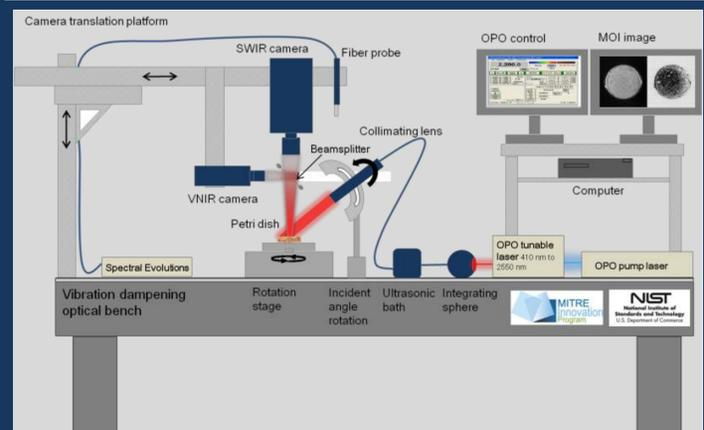
Broad spectral coverage: 405 nm to 2500 nm
