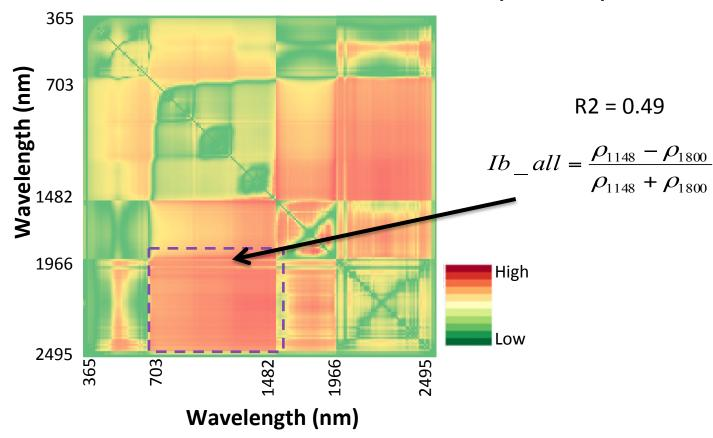
The best band combination is in NIR and SWIR parts of the spectrum
