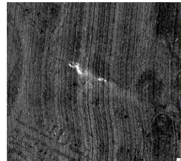
Matched filter reveals plume and highlights plume structure including source transiency and transport induced heterogeneity.
