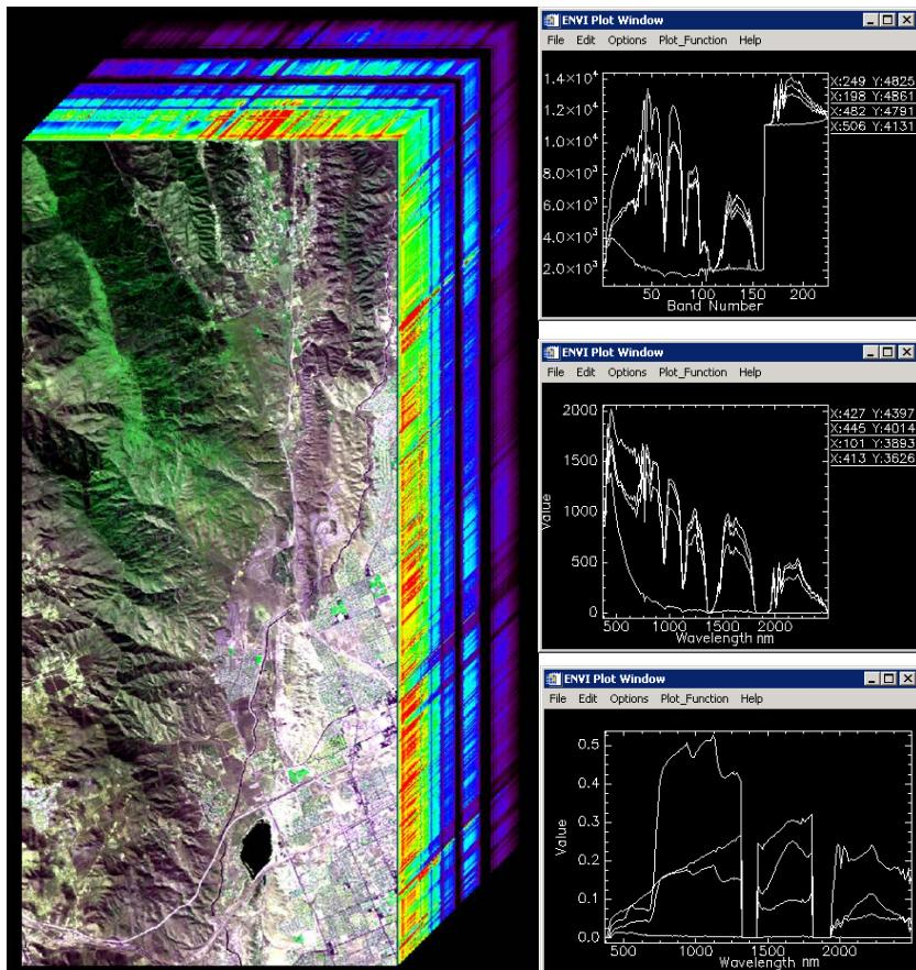
AVIRIS image cube and Level 1a, 1b and 2 spectra. The reflectance spectra (L2) will be used to address the full range of science objectives including ecosystems and climate.
