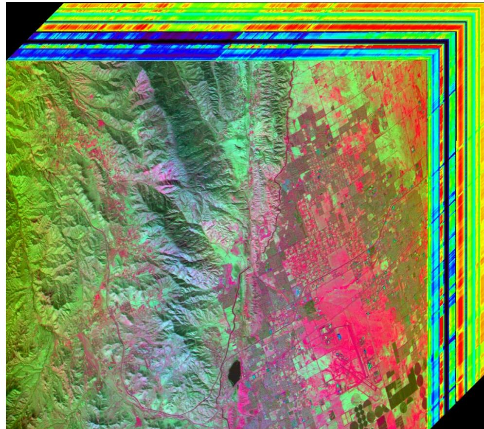
MASTER image cube. Temperature information is shown as color intensity and mimics topography and composition (emissivity) information is shown as color. Red areas are composed of minerals with high silica such as urban areas. Water and heavily vegetated areas are dark indicating they are cooler. HyspIRI temperature and composition information are key to addressing a range of objectives.
