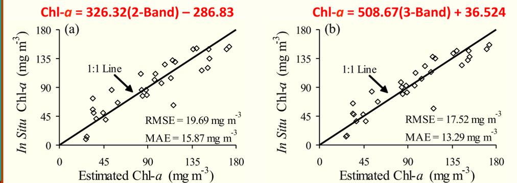
Chl-*a* concentrations measured *in situ* versus chl-*a* concentrations estimated using the HICO-based (a) two-band and (b) three-band NIR-red algorithms, after leave-one-out cross validation.
