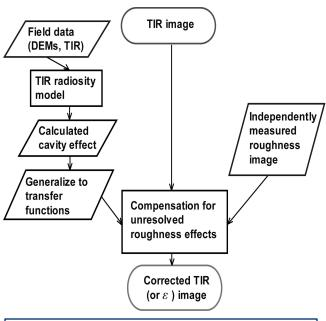
Flow chart illustrating approach to compensation for sub-pixel roughness effects in TIR images.
