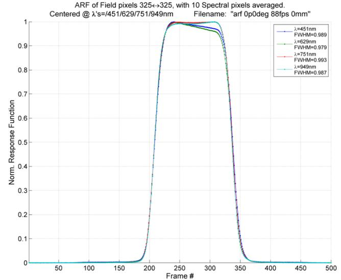
Example along-track spatial response functions (without flight motion blur) for four wavelengths spanning the PRISM spectral range at a single field position.
