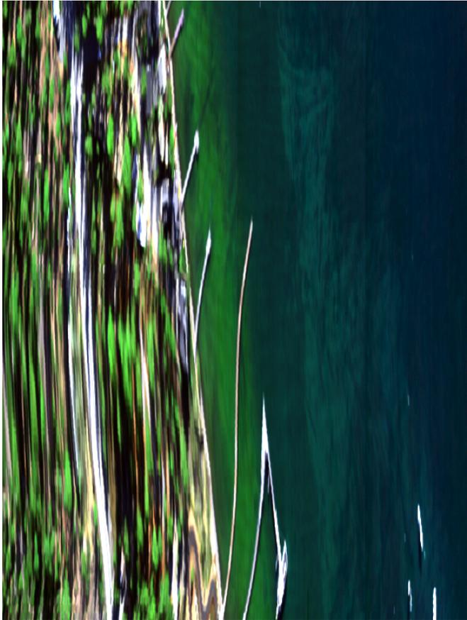
PRISM raw image from Lake Tahoe shows apparent elongation due to along-track oversampling.
