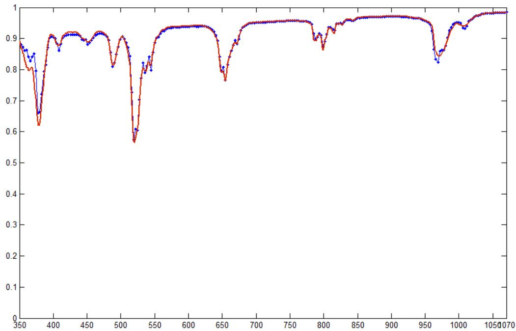
Spectrum of Er-doped spectralon panel received through PRISM (blue curve) and through reference ASD spectrometer (red curve).
