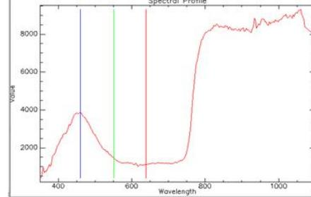
Reflectance after radiometric correction and atmospheric removal
