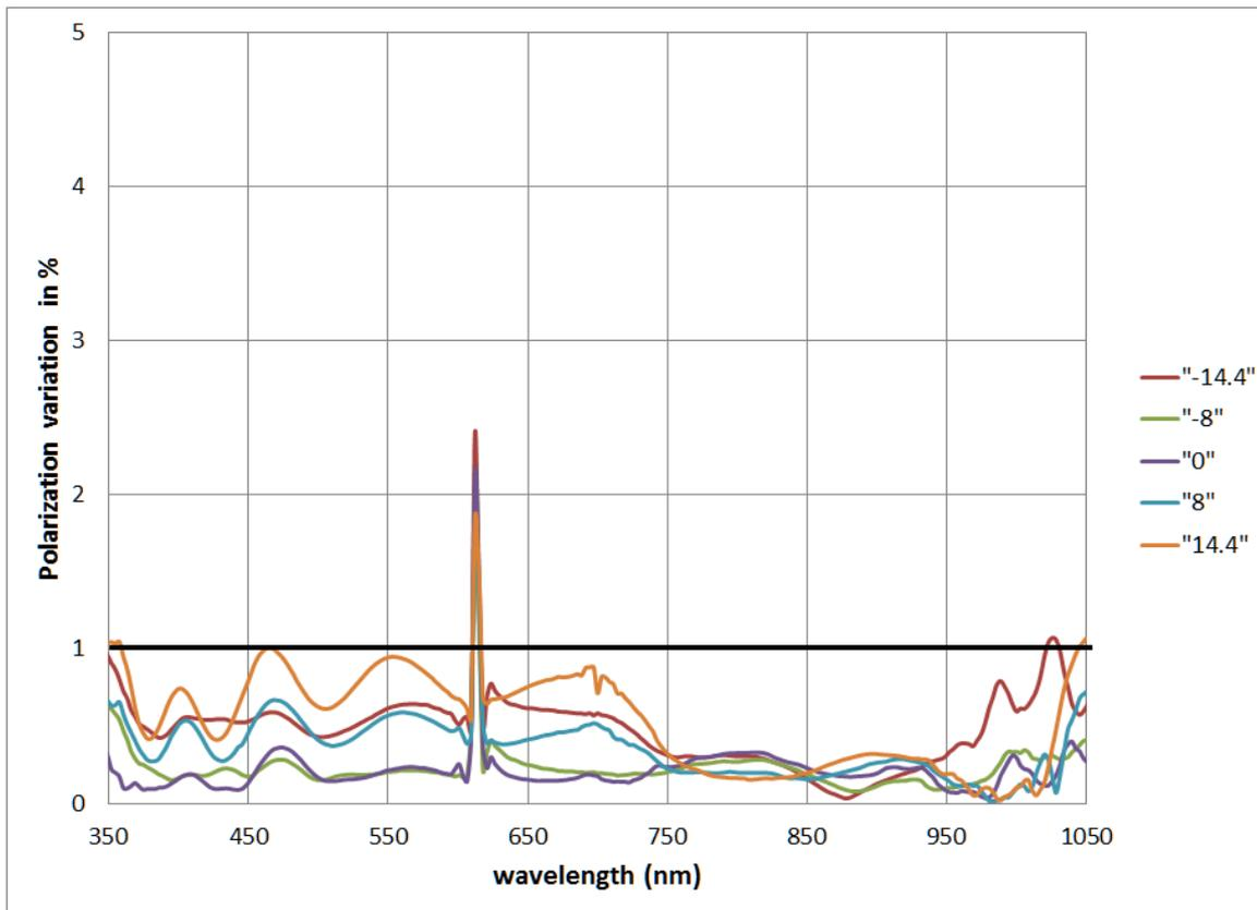
Polarization variation throughout the spectral range for five positions spanning the field of view.
