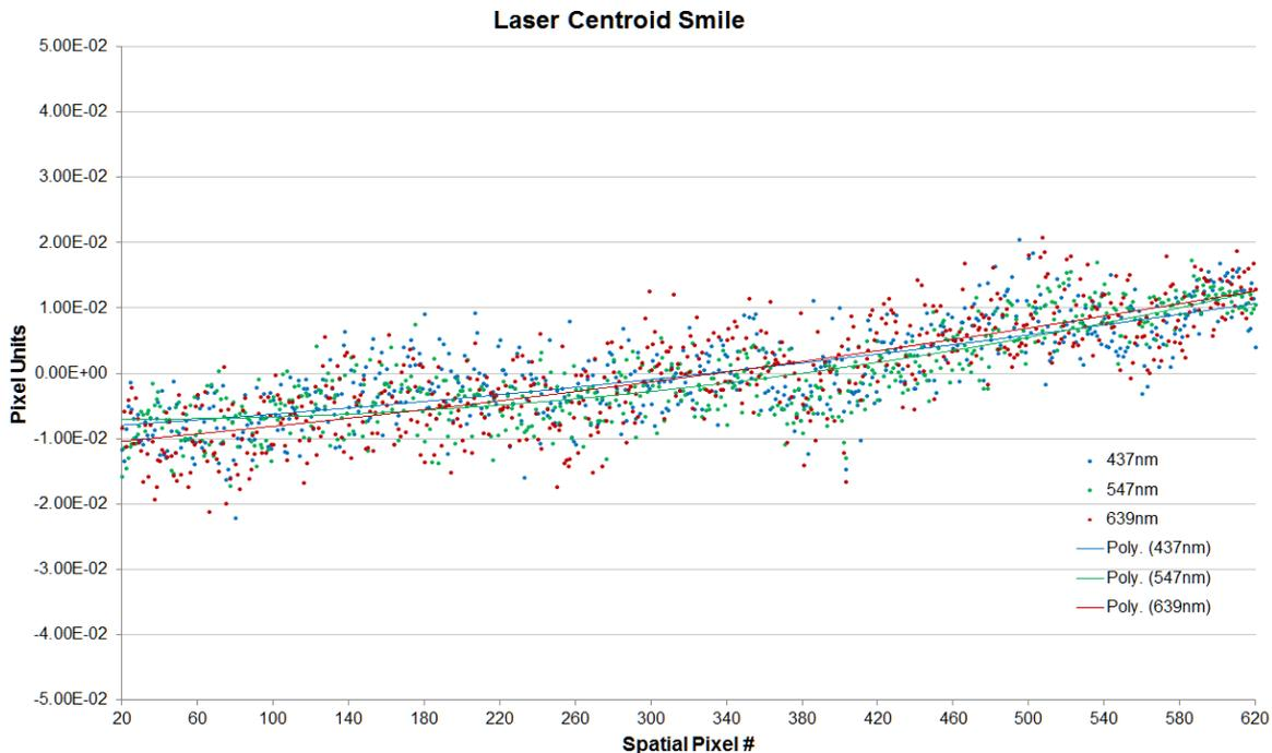
Scatter plot of spectral channel centroids as a function of spatial location for three isolated wavelengths (Hg lamp 437 nm and 547 nm, and laser at 639 nm).
