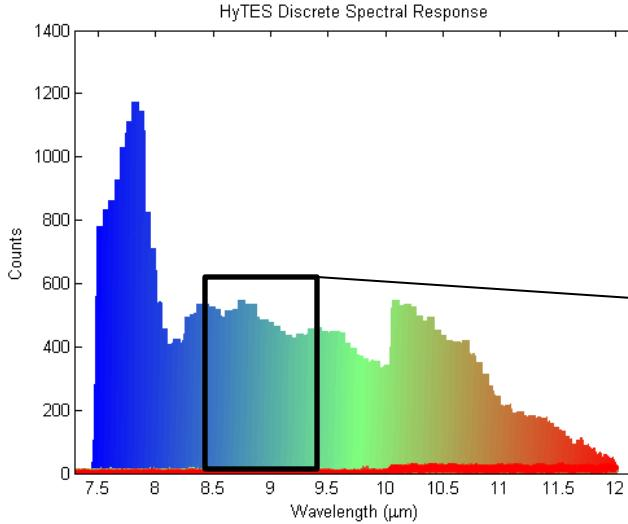
HyTES measured spectral response. A monochromator was cycled through each spectral band while positioned at the entrance aperture.
