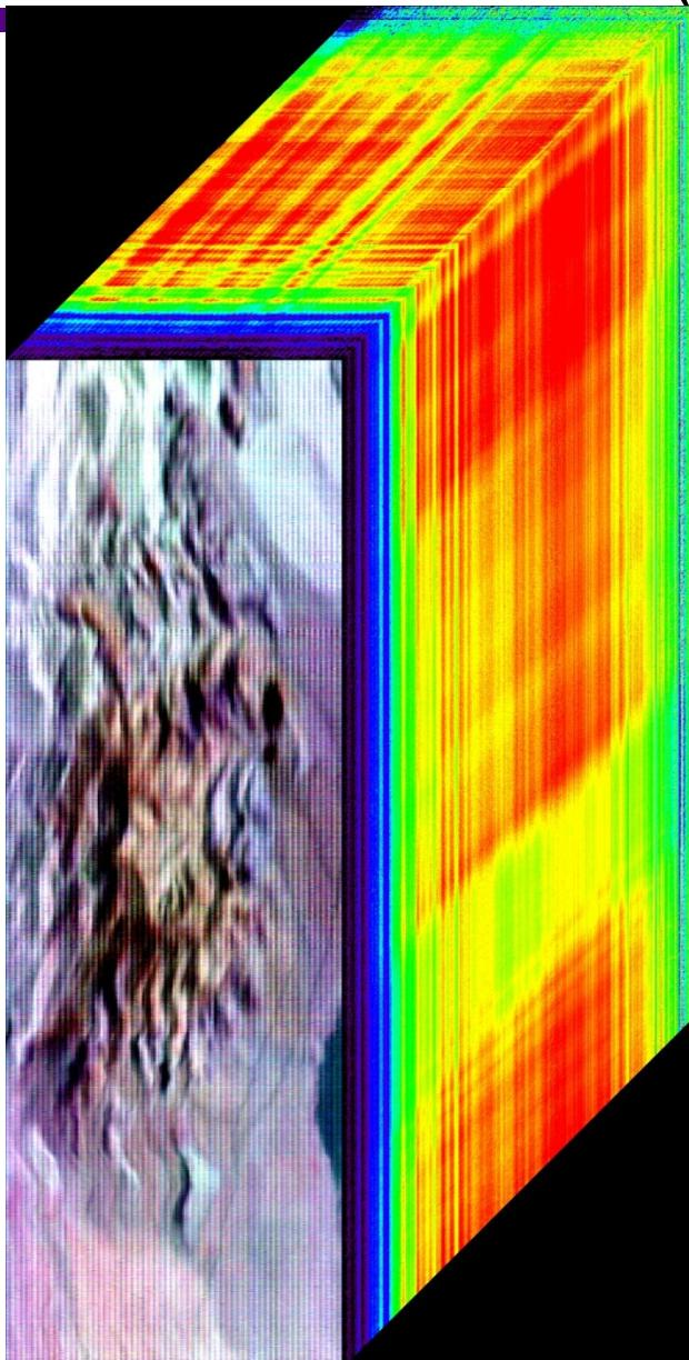
Left: Cuprite, NV 2012-07-20, bands 150 (10.08  $\mu\text{m}$ ), 100 (9.17  $\mu\text{m}$ ), 58 (8.41  $\mu\text{m}$ ) displayed as RGB respectively as image cube.
