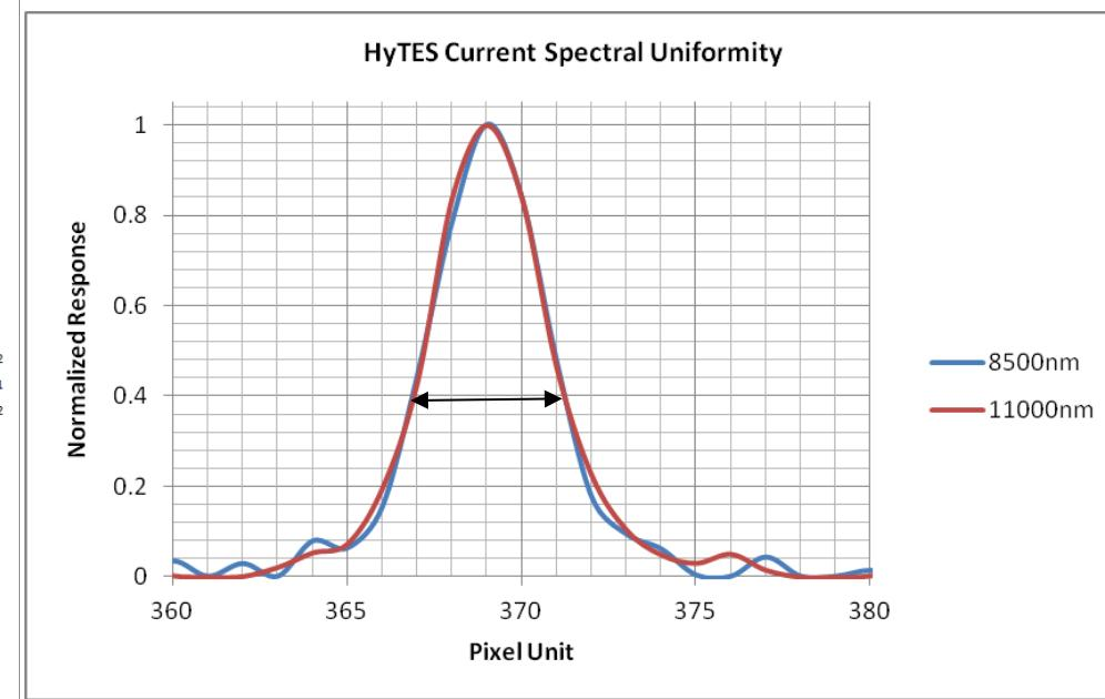
Arrow on measured response shows a FWHM of about 4 pixels (or 2 effective pixels) which is 35.2nm.
