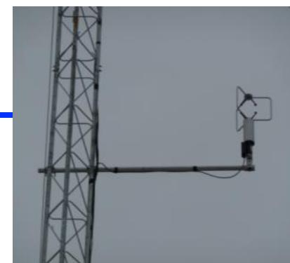
Sub-canopy Flow Sensor at 3m: Sonic anemometer, air temperature, relative humidity and pressure.
