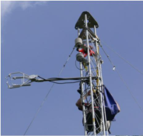
Canopy Flow Sensors at 23 m: Sonic anemometer and gas analyzer, net radiation, air temperature and relative humidity.
