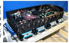
July 2012: Airborne Scanning Microwave Limb Sounder (A-SMLS) – a prototype of a next-generation MLS for measuring trace species in the upper troposphere – completed test flights near Houston, Texas, on the NASA WB-57. A-SMLS successfully acquired ozone measurements and can be configured for a variety of other trace species. (PI: Paul Stek, JPL, IIP-07)
