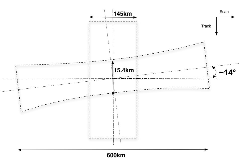
How the VSWIR and TIR would image if TIR bore sight were rotated by ~14°
