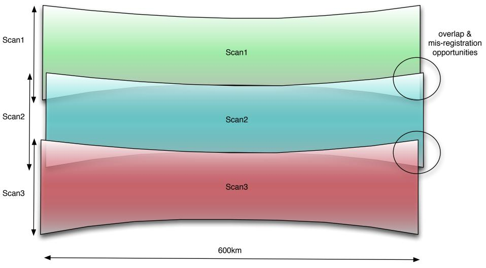
Odd numbered scans are acquired with scan mirror side 1 Even numbered scans are acquired with scan mirror side 2
