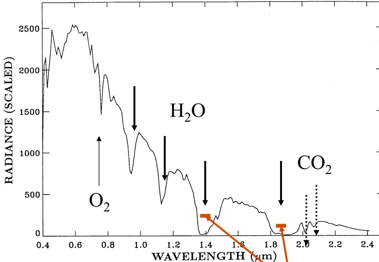
The AVIRIS spectrum is affected by atmospheric absorption and scattering effects. In order to obtain the surface reflectance spectrum, the atmospheric effects need to be removed.
