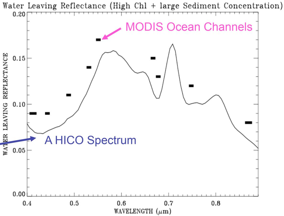
The discrete MODIS ocean channels missed several peaks in the HICO reflectance spectrum. Therefore, MODIS cannot fully characterize the shapes of the spectra acquired over the complex Case 2 waters.
