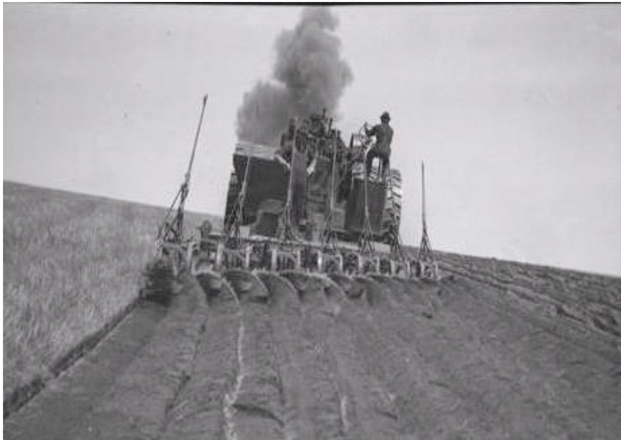
Steam plow breaking native prairie in early 1900s in ND. Institute for Regional Studies, NDSU.
