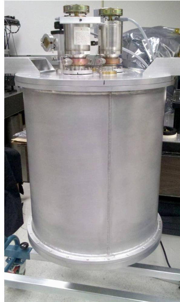
Spectrometer housing and Relay Assembly
