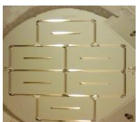
Ultra uniform 27  $\mu\text{m}$  x 20 mm electron-beam lithography slit for space flight
