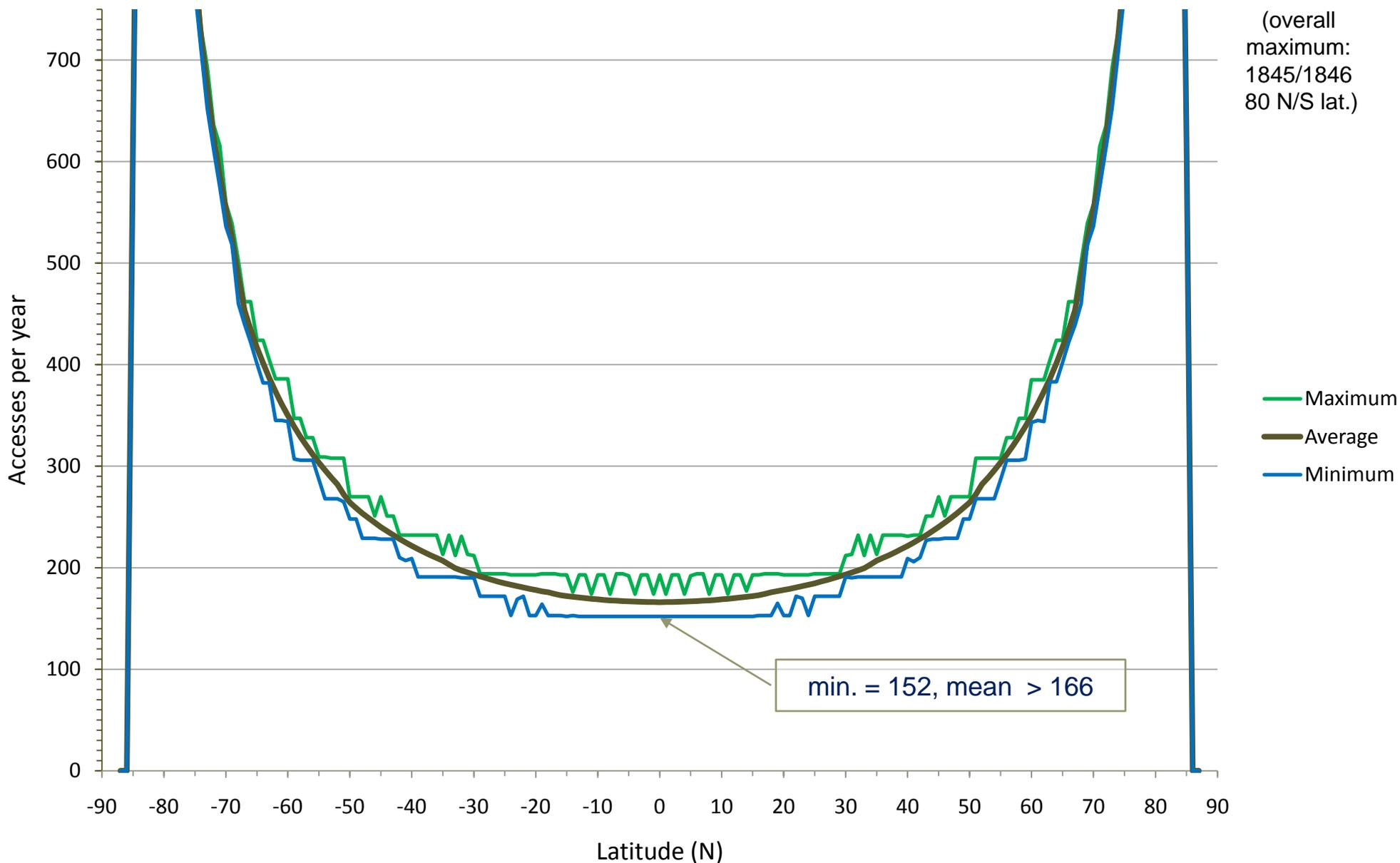
Nominal orbit: average alt. 626.8 km, inclination 97.8°. TIR imager FOV: +/- 25.46° (60 m pixel GSD at nadir, 9272 cross-track pixels).
