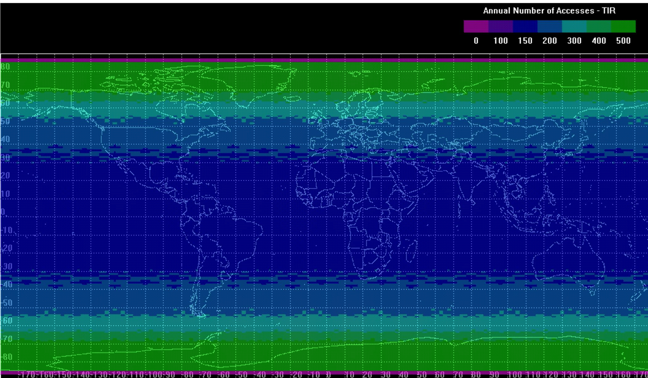
Nominal orbit: average alt. 626.8 km, inclination 97.8°. TIR imager FOV:  $\pm 25.46^\circ$  (60 m pixel GSD at nadir, 9272 cross-track pixels).
