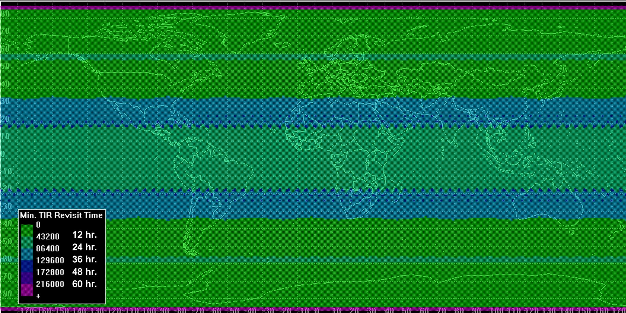
Nominal orbit: alt. 626.8 km, incl.: 97.8. TIR sensor FOV: +/- 25.46 (60 m pixel GSD at nadir, 9272 cross-track pixels).
