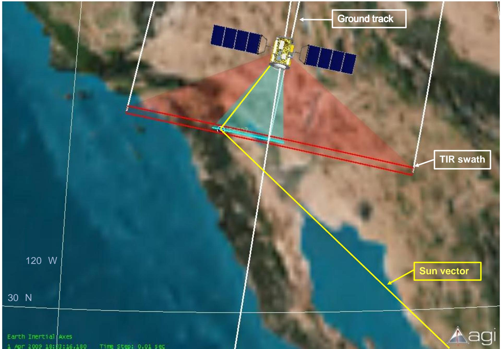
VSWIR swath (light blue) is nested within TIR cross-track scan pattern (red), with a swath center offset west of the satellite's ground track (white). Note view & illumination vectors (yellow). Access geometry simulated for 1 Apr 2009, 18:33:16.18 UTC, with STK v9.2.
