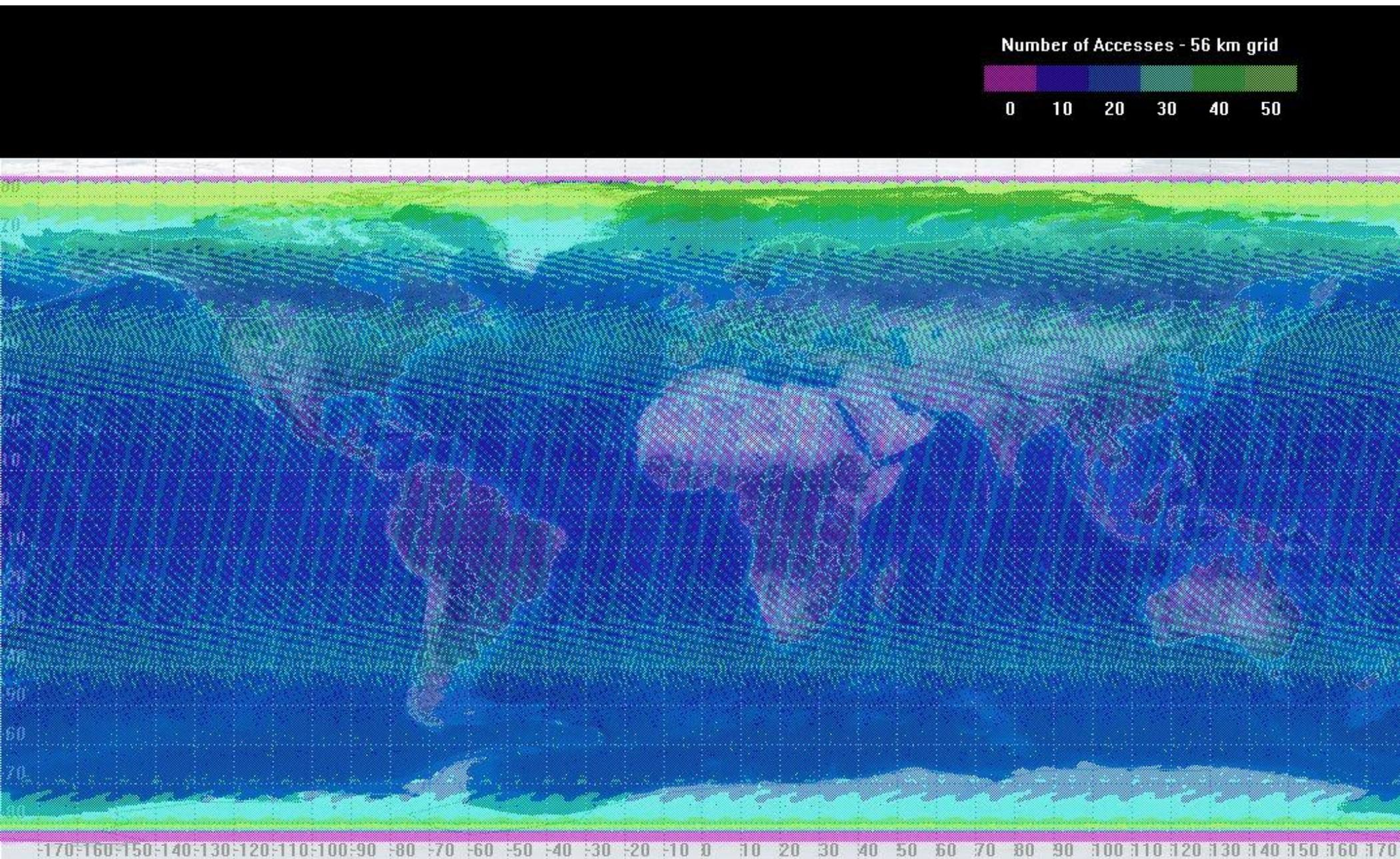
Nominal orbit: av. alt. 626.8 km, incl. 97.8°. VSWIR spectrometer FOV: 2.8° E, 10.8° W (60 m pixel GSD at nadir, 2480 cross-track pixels).
