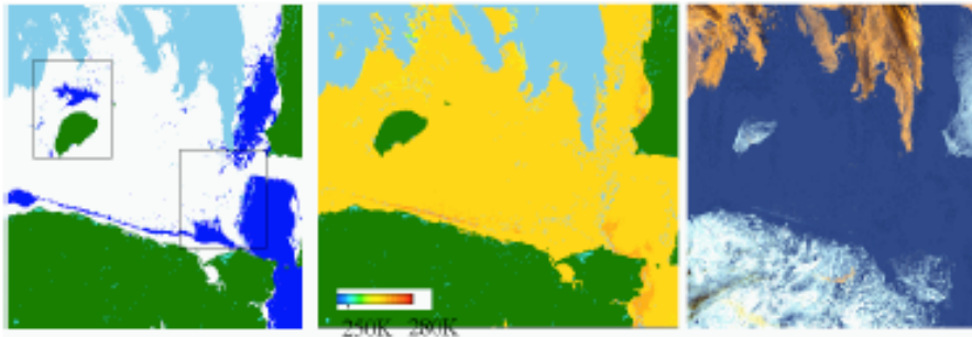
Figure 4: MODIS sea ice product by NDSI method (left), IST method calculated temperatures (center), and a composite image made from MODIS Bands 20 ( 3.7\mu\text{m} ), 22 ( 3.9\mu\text{m} ) and 23 ( 4.0\mu\text{m} ) to highlight clouds (right).
