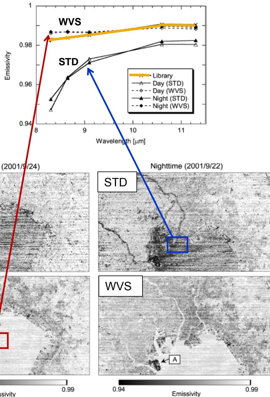
Fig. 20. Emissivity maps of band 12 retrieved from the daytime and nighttime scenes by each method.
